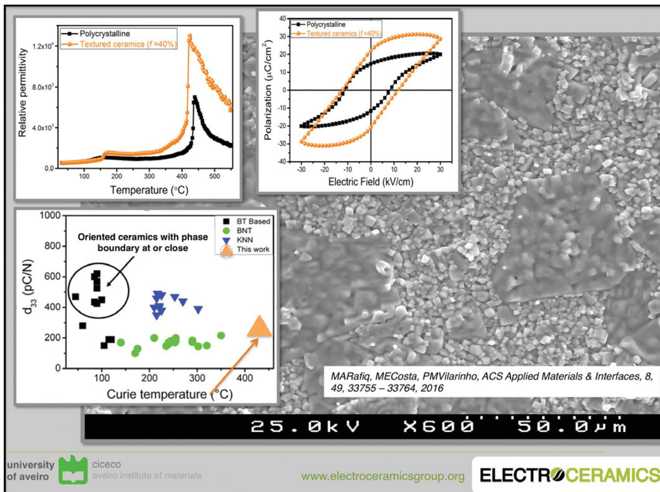
Fig. 2 Pairing high piezoelectric coefficient  $d_{33}$  with high Curie temperature ( $T_c$ ) in lead-free  $(K,Na)NbO_3$ . Adapted from reference 5
