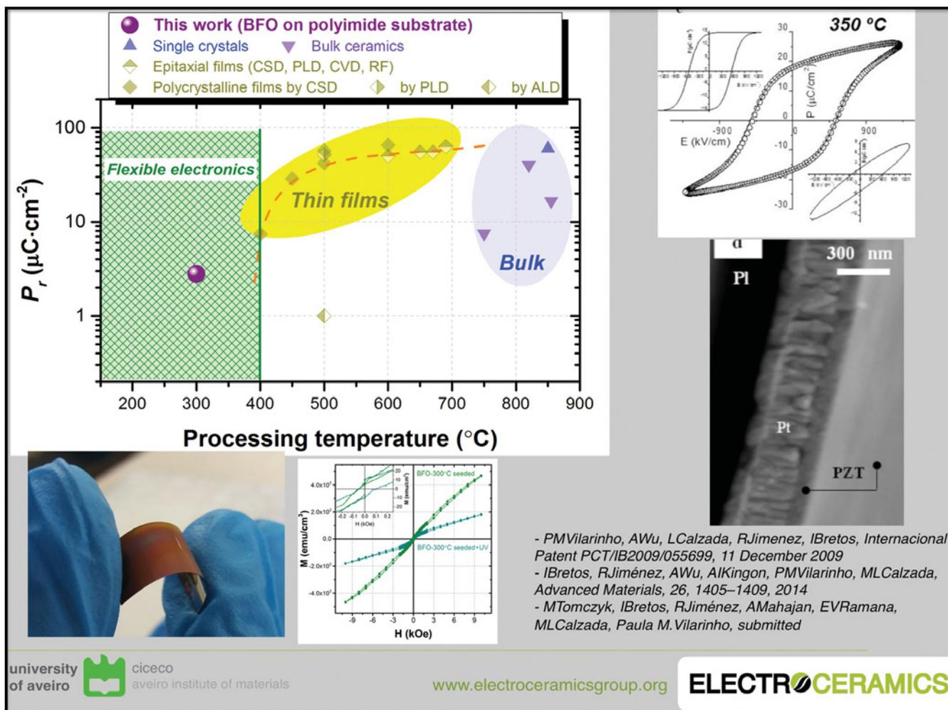
Fig. 1 Direct fabrication of  $PbZr_{1-x}Ti_xO_3$  and  $BiFeO_3$  thin films on polyimide substrates for flexible electronics. Adapted from reference 3 and 4
